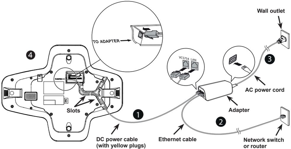
1. Plug one end of the DC power cable into the power jack of the base unit, and plug the other end into the **VCS754** jack of the power adapter. Route the cord through the slots.
