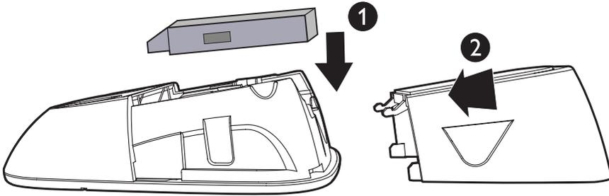
1. Place the battery (with the label **THIS SIDE UP** facing up) into the battery compartment.
